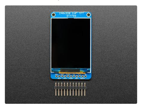
The breakout has the TFT display soldered on (it uses a delicate flex-circuit connector) as well as a ultra-low-dropout 3.3V regulator, auto-reset circuitry, and a 3/5V level shifter so you can use it with 3.3V or 5V power and logic. We also had a little space so we placed a microSD card holder so you can easily load full color bitmaps from a FAT16/FAT32 formatted microSD card. The microSD card is not included, but you can pick one up here (http://adafru.it/102).
