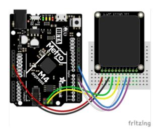
Vin connects to the Metro's 5V or 3.3 pin. GND connects to any one of the Metro's Gnd pins.
