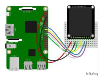
Vin connects to the Raspberry Pi's 3V pin GND connects to the Raspberry Pi's ground
