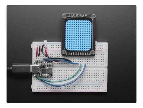
Don't be such a square - throw a curve-ball into your electronics with a curved-edge miniature display. Here's a new "round rect" TFT display - it's 1.69" diagonal and has a high-density 220 ppi, 280x240 full color pixels with IPS any-angle viewing.
